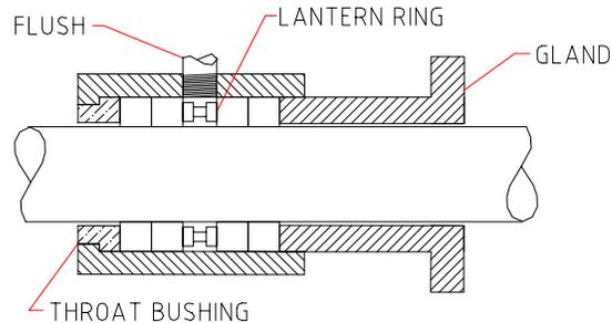
Because compressed, stacked packing requires leakage to cool and lubricate, one would normally use packing on benign products. If used on environmentally unfriendly products or dangerous goods, the leakage must be collected and suitably treated to protect people and environment. Graphite impregnated shaft packing is self-lubricating and reduces wear on the shaft.
