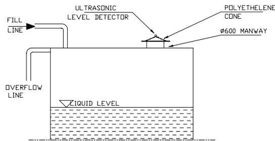
Figure No. 2. Ultrasonic level detector in a flat top roof
