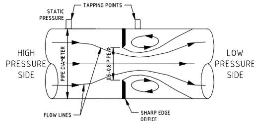
Figure No. 1. Orifice Plate Flow Meter.
