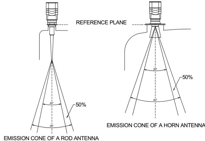
FIGURE 1 Rod and horn style radar detectors
